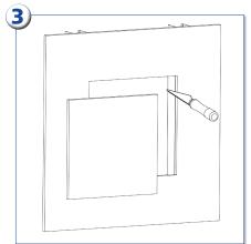
Measure the outer dimensions of the panel. Mark the panel measurements.
